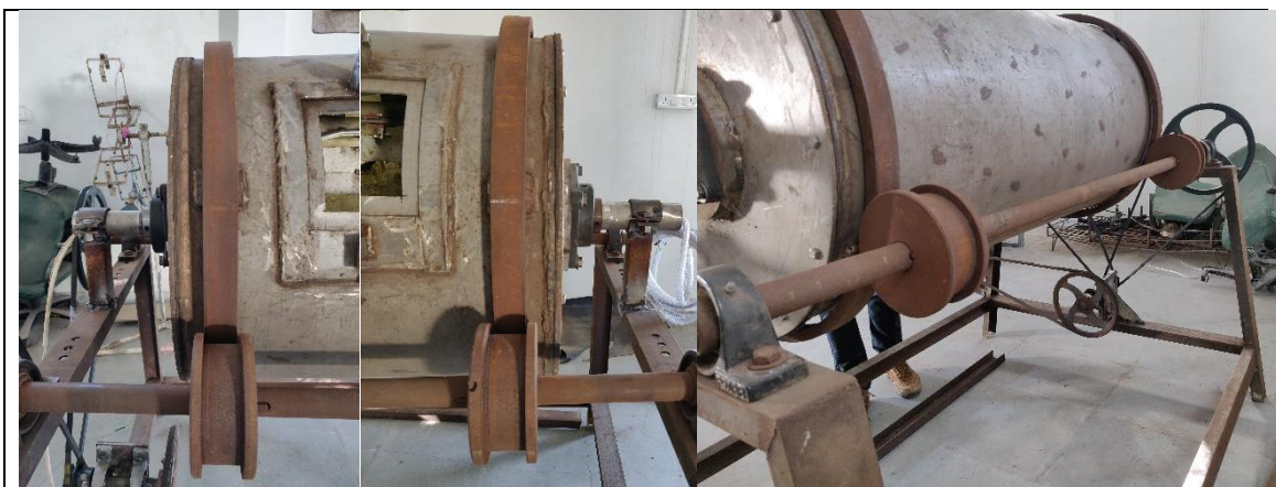
Plate 3.5 Fitting of rollers to support the drum
