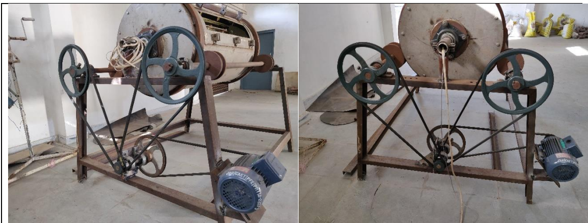
Plate 3.10 Fitting of electric motor and driving mechanism to rotate the drum
