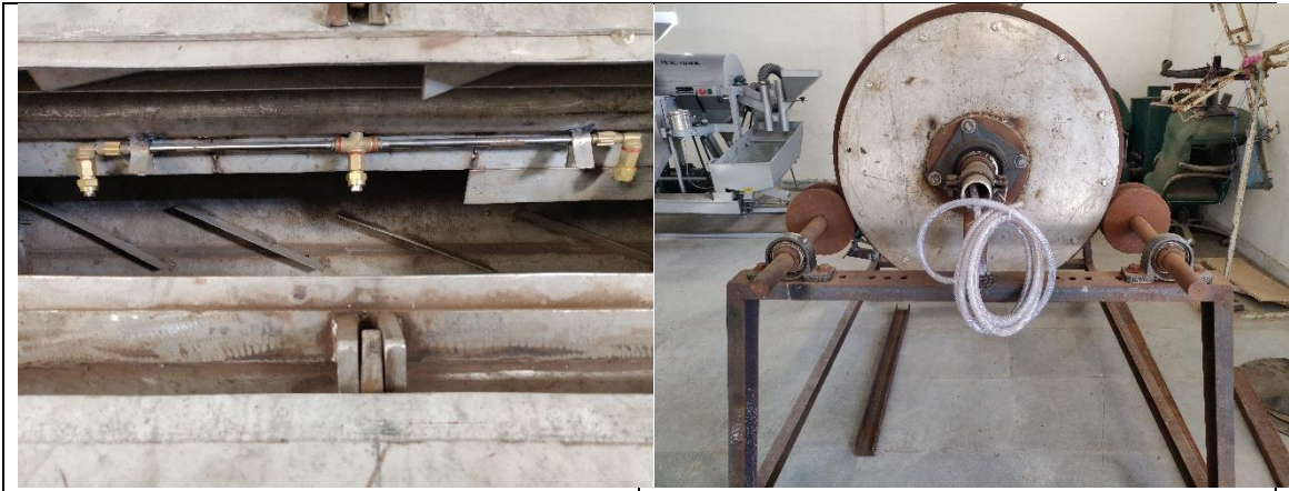
Plate 3.8 Fitting of spray nozzles inside the drum
