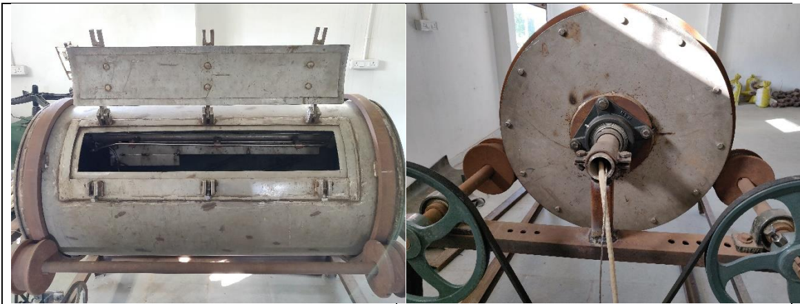
Plate 3.9 Fitting of heater assembly inside the drum
